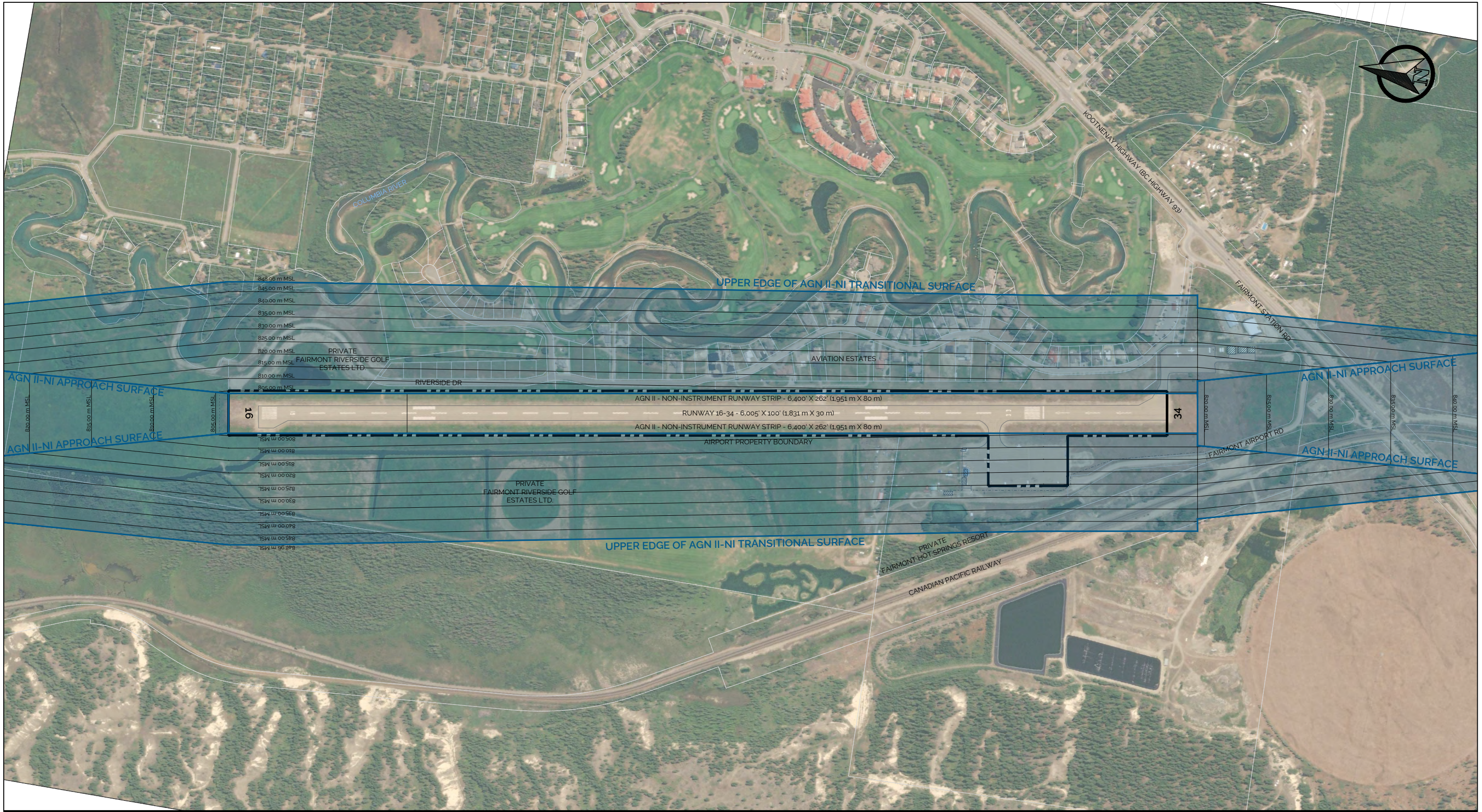
COLUMBIA VALLEY AIRPORT AT FAIRMONT HOT SPRINGS AIRPORT MASTER PLAN FIGURE 6.1 - OBSTACLE LIMITATION SURFACES NOVEMBER 2023
